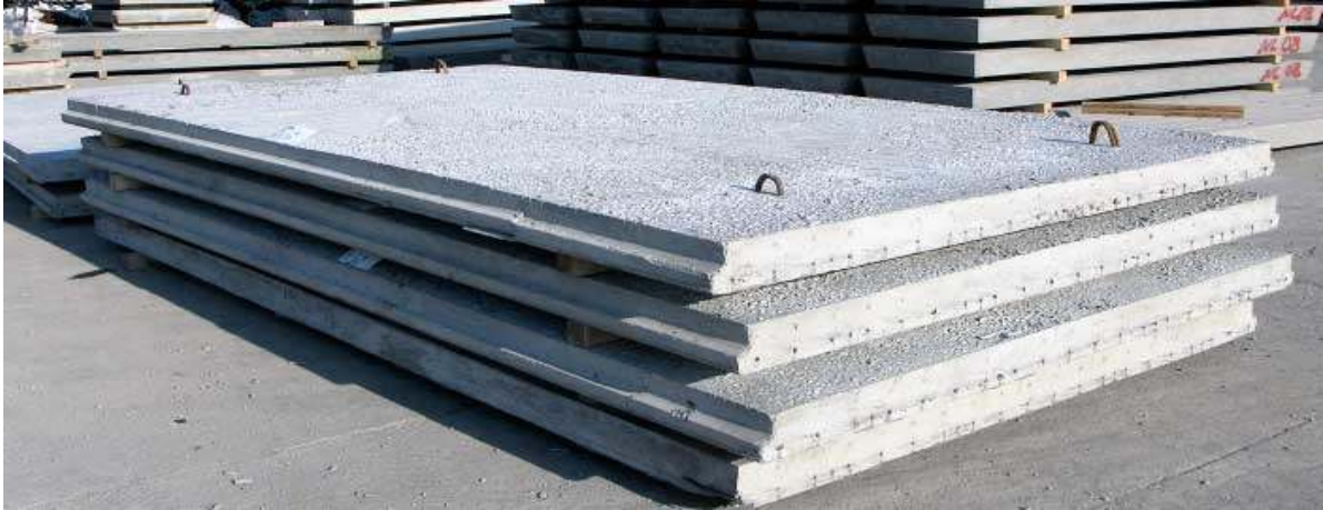
Fig: Prestressed solid slabs
