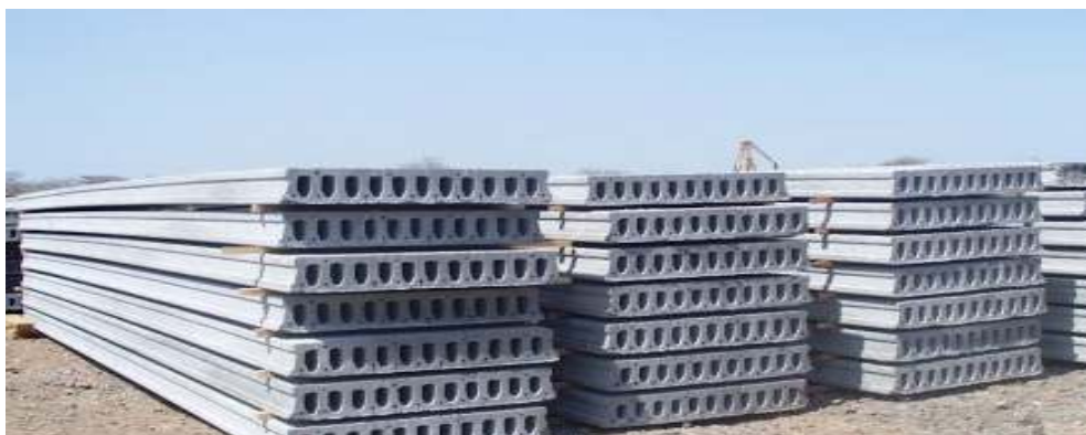
Fig: Prestressed hollow core slabs
