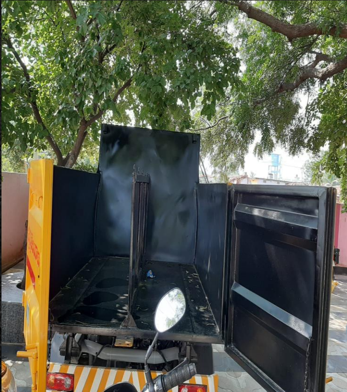
Garbage collector with separation of dry and wet waste
